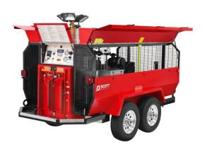
The easy-tow Liberty II breathing air system is a totally enclosed dual axle trailer that is well suited for mobile applications. It comes with four ASME storage cylinders, Scott Safety RevolveAir charge station, Scott Safety X4 controller/monitor (monitors CO & Dew Point) for safety operation, and is capable of being towed by any vehicle rated for 7,000 GVW or more.
