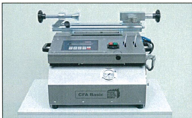
Fig. 2: Space saving placement of the Basic Digital supplementary unit directly on top of the CFA Basic pump unit.
