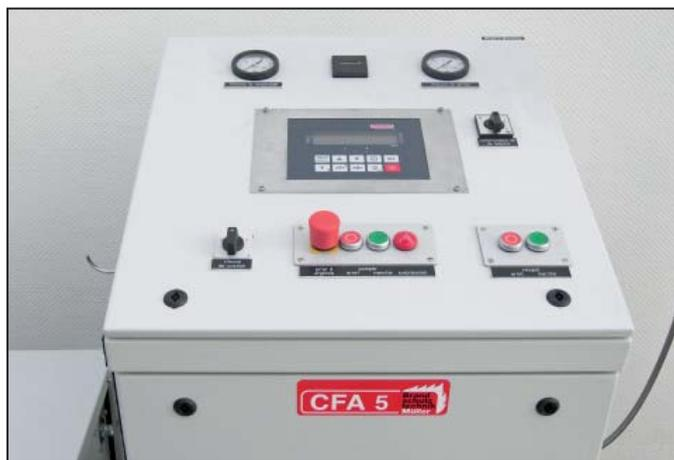
Fig. 3: The control stand is ergonomically designed to ensure comfort and convenience during operation. It contains displays for weight on the scales, filling pressure, circulating initial pressure, excess pressure control and an operating hour counter. 3 different freely programmable cut-out weights can be called up for the scales with a selector switch.
